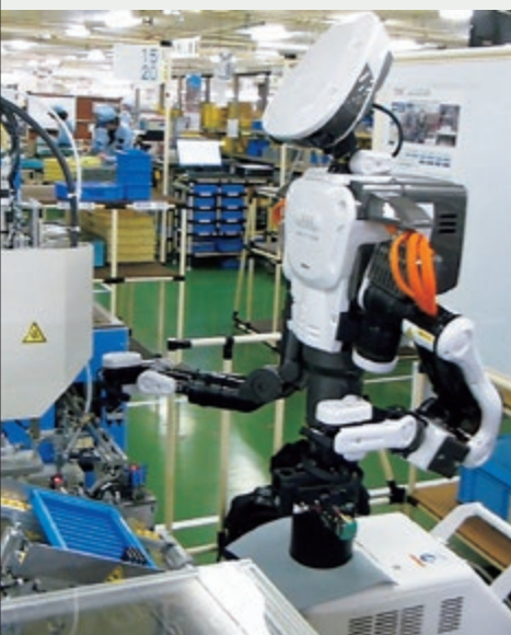
NEXTAGE® performing assembly work at the YAMAGATA Plant
