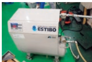
Electric booster compressor
