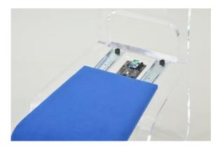
Slide rails built into the seat of the chair are used to pull the seat back to load or remove a microcomputer.
