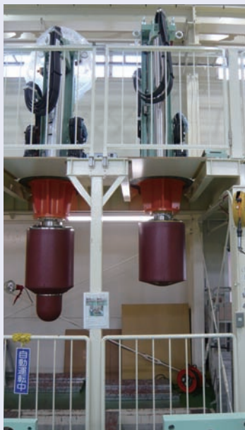
Rolling mechanism used in internal vertical-motion component. The red portions are the sensors.
