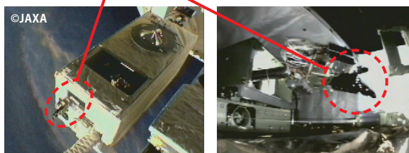
Robotic hand used at the International Space Station experiment module.
