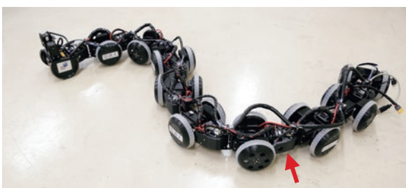
The T2 Snake-3 features a SEED MS on the side of each joint (indicated by the arrow)
