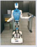
The thermometric robot keeps its left arm up when a body temperature exceeds a certain amount
