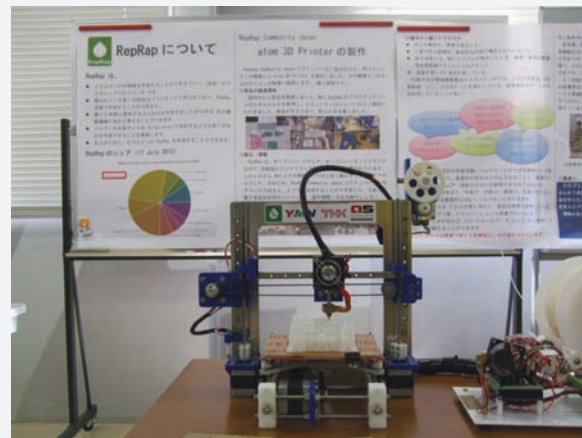
A 3-D printer incorporating THK products.
