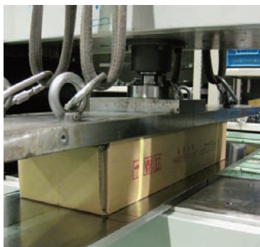
Testing a packing box's pressure-tolerance.
