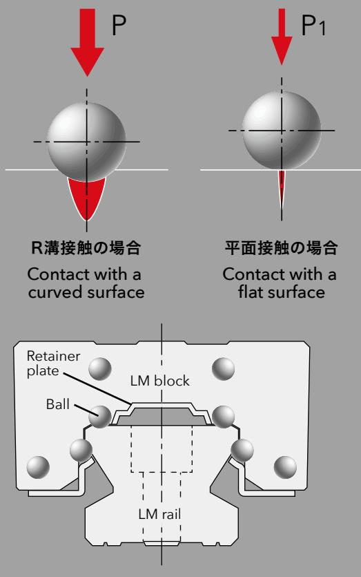
Caged ball technology was developed as a result of combining THK's technology and expertise. This technology, which enables higher precision and service life in linear motion systems, does not simply improve mechanical performance, but also prevents the accumulation of dust particles and reduces required maintenance. It adds to the energy efficiency of linear motion systems, helping us make strides in developing eco-friendly products.
