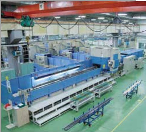
7-meter grinding machine for LM rails
