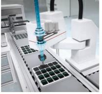
Horizontal articulated robot (SCARA robot)
