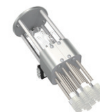
Adaptive Suction Hand The built-in flow restrictor accommodates for suction error.
