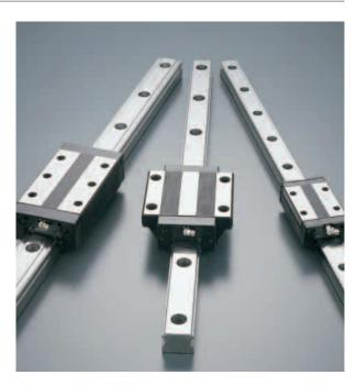
LM guides with cage-embedded technology contain belt-shaped ball cages that hold the balls in place while preventing contact between them. This design translates into benefits such as extended service life, reduced noise and less generation of heat and dust, thus reducing overall costs for customers.
