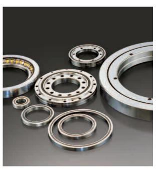
Cross roller rings feature internal cylindrical rollers arranged orthogonally to facilitate load bearing in every direction.
