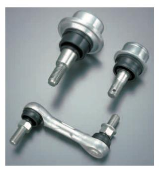
Use of an integral molding process for the aluminum die-cast produces lightweight link balls that are highly resistant to corrosion and abrasion. These are used widely in vehicle undercarriages.
