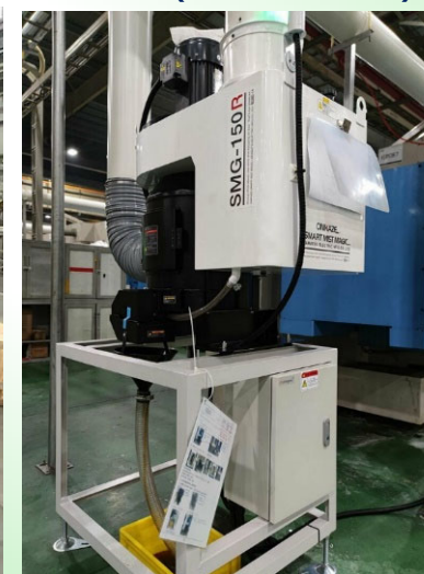
An inverter function was added to the mist collectors (THK Wuxi Plant)
