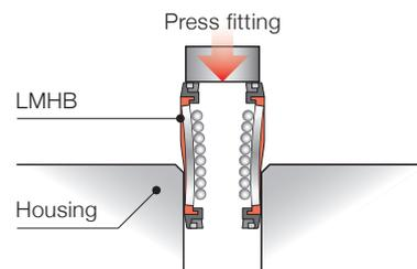
\* A snap ring, stop plate, or other fastener can be installed to further improve the pull-out strength of the housing.
