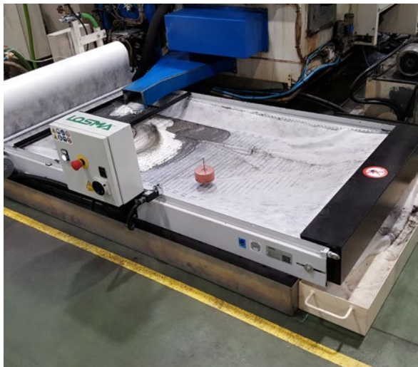
Metal shavings and grains are now filtered and stay on top of the paper
