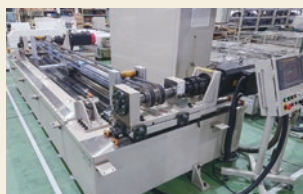
LM Guide high-speed durability tester
