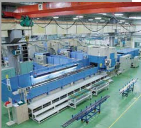
7-meter grinding machine for LM rails
