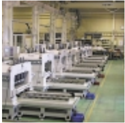
Durability testing devices for determining reliability of LM guides
