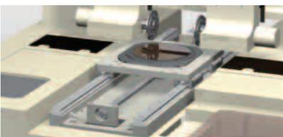
Ball screw used in a dicing saw (for semiconductor production)
