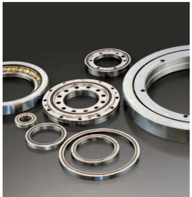
Cross roller rings feature internal cylindrical rollers arranged orthogonally to facilitate load bearing in every direction.
