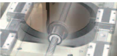
Application of ball screws and LM guides
