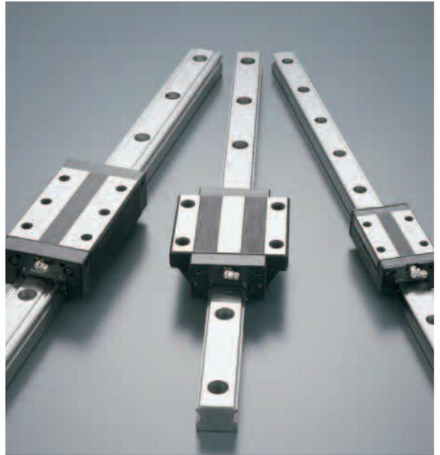
LM guides with cage-embedded technology contain belt-shaped ball cages that hold the balls in place while preventing contact between them. This design translates into benefits such as extended service life, reduced noise and less generation of heat and dust, thus reducing overall costs for customers.
