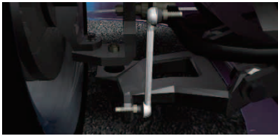
Application of link balls
