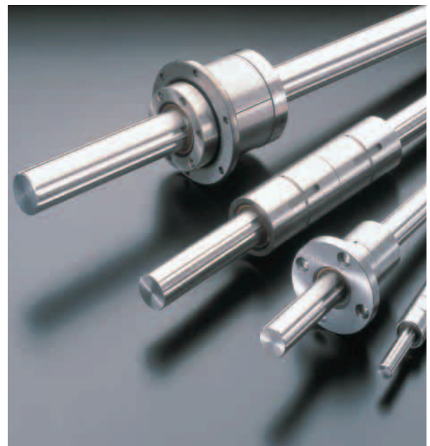
Ball splines are devices in which balls embedded in the spline nut are allowed to move smoothly along a precision-machined groove in the rolling surface of the spline axle. This design creates a linear-motion system that is capable of transmitting torque.
