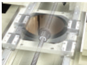
Ball screw used in a dicing saw (for semiconductor production)
