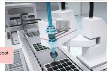
Horizontal articulated robot (SCARA robot)
