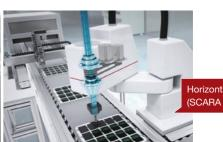
Horizontal articulated robot (SCARA robot)
