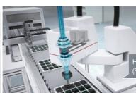
Horizontal articulated robot (SCARA robot)
