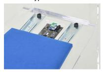
Slide rails are built into the seat of the chair that are used to pull the seat back to load or remove a microcomputer.
