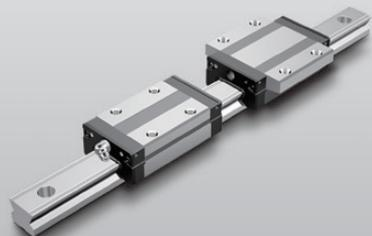
Radial Type design placed the Balls at 90° contact angle, best fit for horizontal applications. Caged Ball technology enables longer service life and noise reduction.
