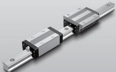
Each row of Balls placed at a contact angle of 45°, allows usage in all orientations. Caged Ball technology enables longer service life and noise reduction.
