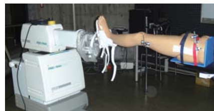
④ Repositioning robot assisting a surgical procedure
