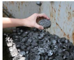
▲ Solidified sludge at the KOFU Plant
